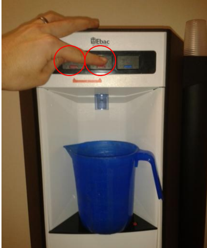
Dispense 3 liters of water from the Hot side by pressing the buttons above
